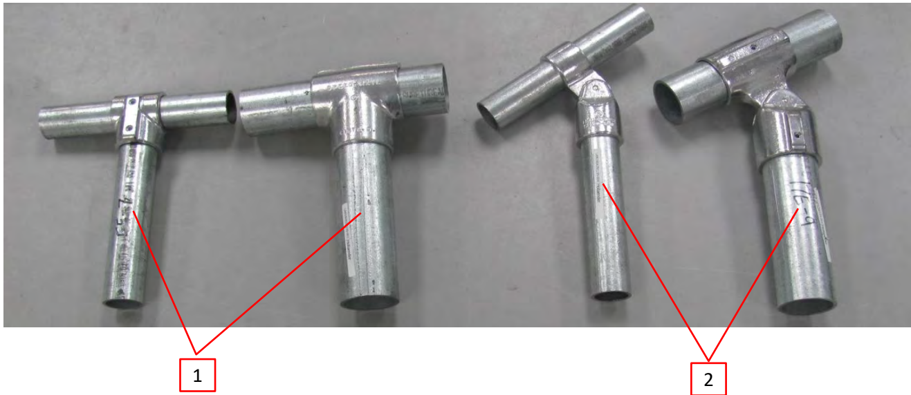
Photo 1 - Tee Fittings (two from left) and Adjustable Brace Fittings (two from right)
